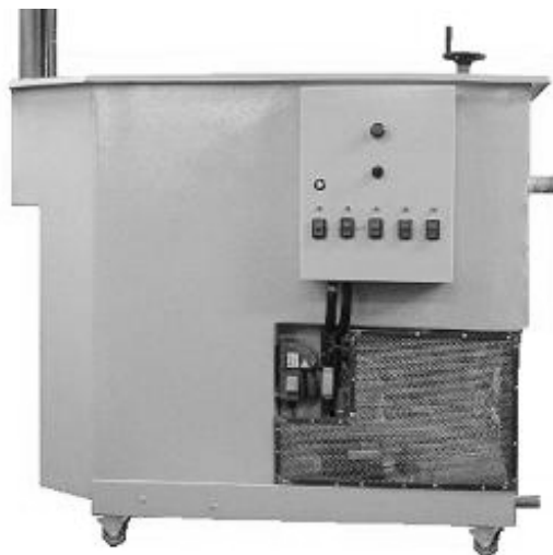
Figure 9. FF pilot system used in the removal of oils from oil-in-water emulsions.
